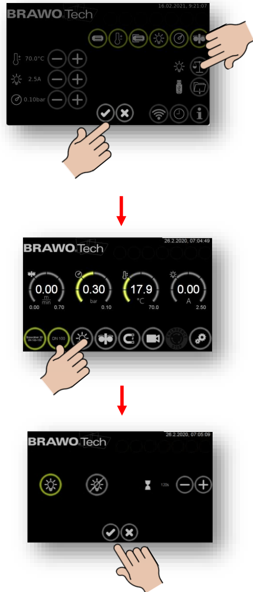
Figure 49 Calibrating the current consumption of the LED head
