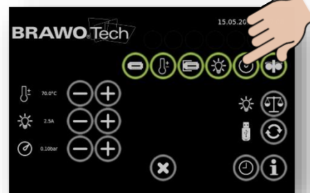
Figure 86 Switch on working pressure monitoring
