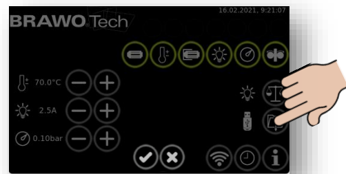
Figure 50 Download LED head current consumption
